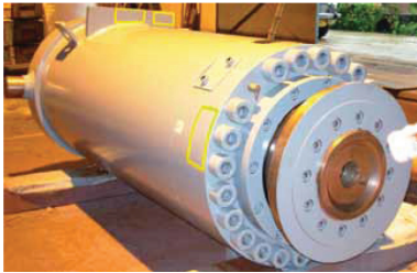
Ladle lifting & tilting hydraulic cylinder having bore dia 500 mm with ceramic coated plunger for continuous casting shop
