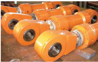
Double acting hydraulic cylinders fitted with heat resistant bellow for walking beam furnace application
