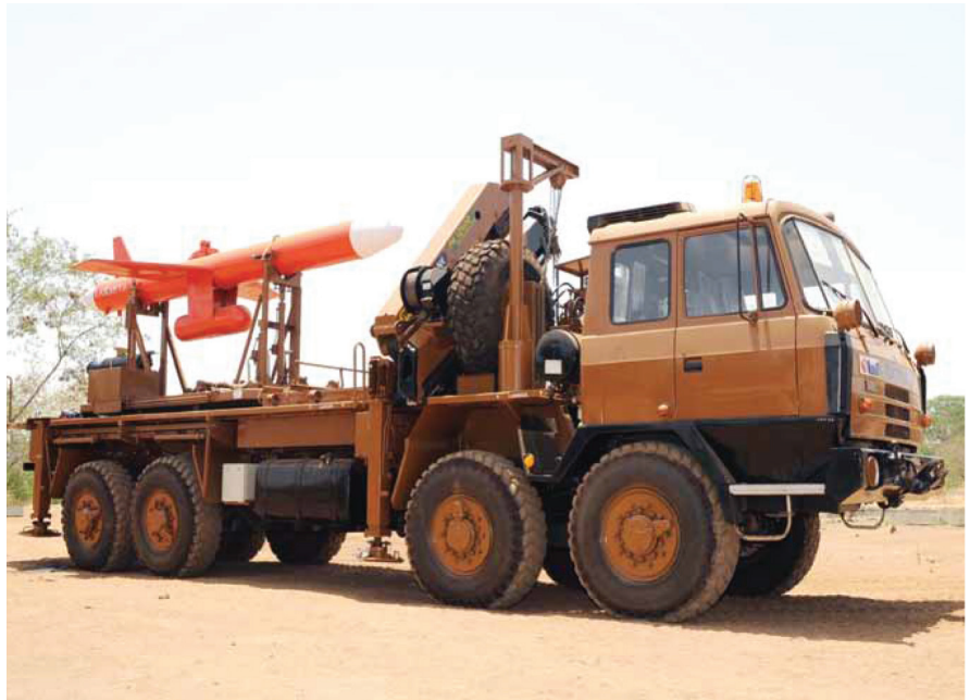
Manufacturing of Pilotless Target Aircraft (PTA) launcher including complete hydraulic system and controls – Project Lakshya
