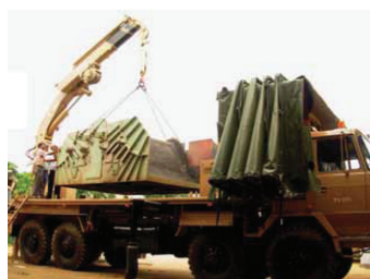
Manufacturing of Jet Deflector Carrier Equipment and installation of the same on Tatra Chassis along with 30 MT crane along with complete hydraulic system
