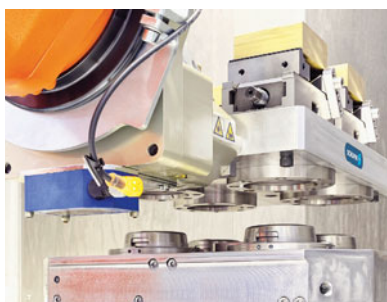
The four clamping rings rest flush on the outer diameter of the quick-change pallet module. This ensures ideal support for transmitting high torques
