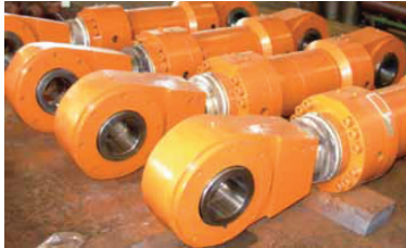
Double Acting Hydraulic Cylinders fitted with Heat Resistant Bellow for Walking Beam Furnace application.
