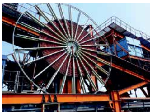
Cable Reeling Drums
