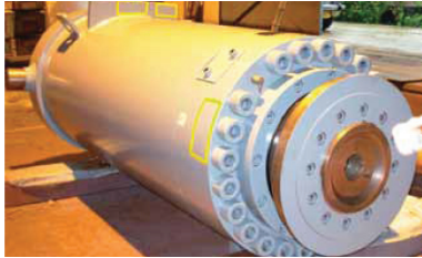
Ladle Lifting & Tilting Hydraulic Cylinder having Bore Dia 500 mm Bore with Ceramic Coated Plunger for Continuous Casting Shop.
