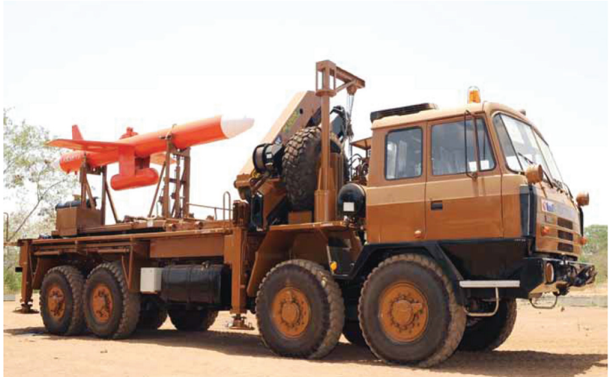
Manufacturing of Pilotless Target Aircraft (P.T.A.) Launcher including complete Hydraulic System and Controls. – Project Lakshya.
