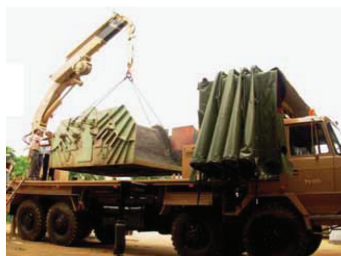
Manufacturing of Jet Deflector Carrier Equipment and installation of the same on Tatra Chesis along with 30 MT Crane along with complete Hydraulic System
