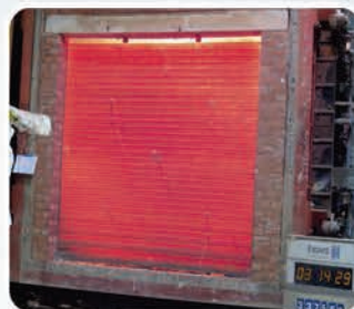
AFTER 3 hrs FIRE TESTING
