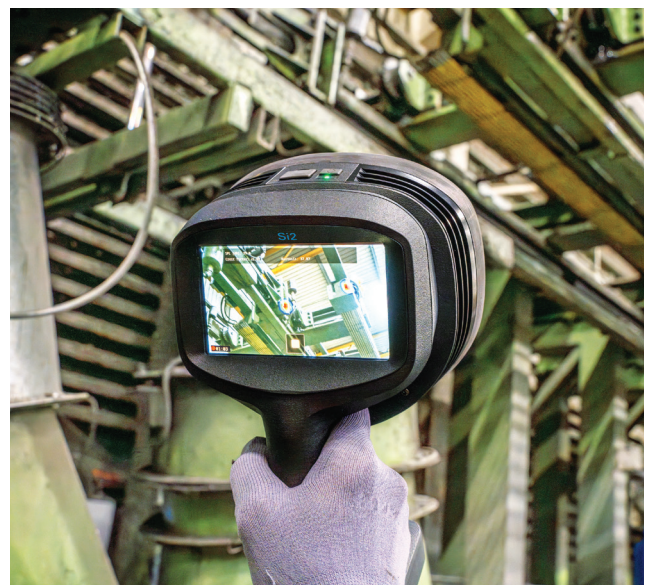
The FLIR Si2-LD detects two sources of potential compressed air leaks, distinguished from background noise.
