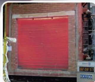
AFTER 2 hrs FIRE TESTING
