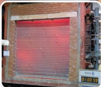
AFTER 1 hr FIRE TESTING
