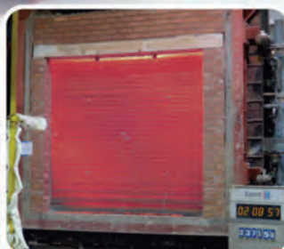
AFTER 2 hrs FIRE TESTING
