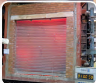
AFTER 1 hr FIRE TESTING
