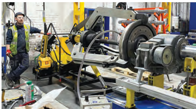
Removing a wheel shaft with the Enerpac LGH3100 100-ton Lock-Grip Puller.
