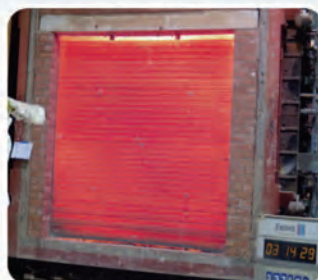
AFTER 3 hrs FIRE TESTING
