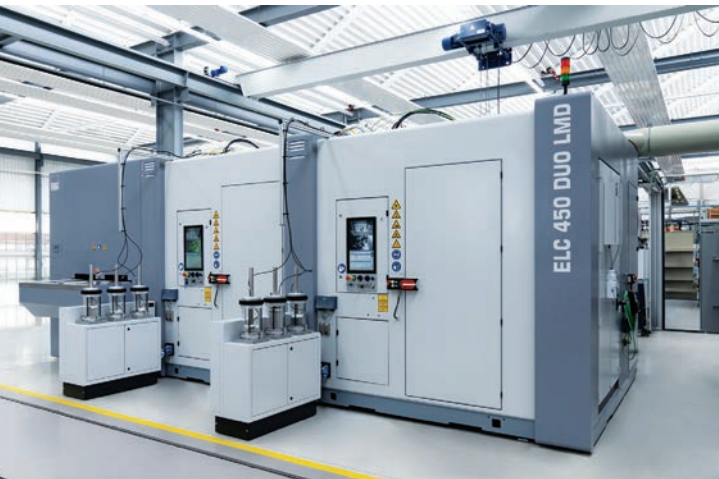
EMAG's ELC 450 DUO LMD with two process modules enables increased productivity in the hard coating of brake disks.
