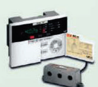
Intelligent Motor Controller [0.125~60A]
