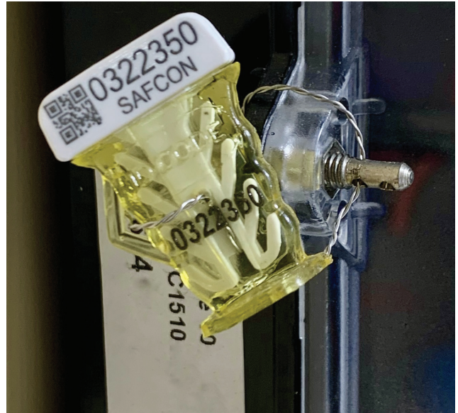
Meter seal with male and female parts pre-locked
