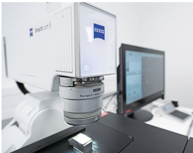
Magnification of the fracture surface with the digital microscope ZEISS Smartzoom 5.
