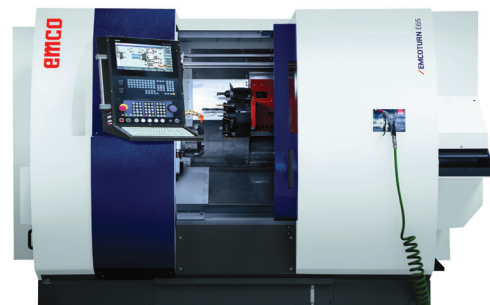
The CNC turning centre EMCOTURN E65 primarily produces screw cores for GF Casting Solutions. This makes it possible to produce spare parts at a high level and at high speed.
