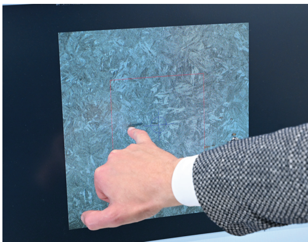
The analysis confirms contamination on the central axis; non-metallic inclusions from foreign material are also detected.
