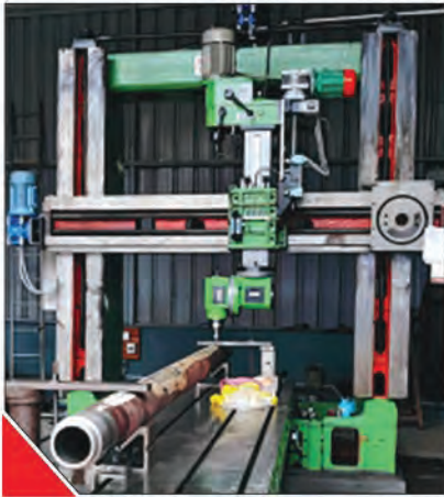
Ram Type Milling Head In Combination With Spherically Contouring Universal Milling Head Adds Linear & Multi Angle Machining Capability To An Old Planer.
