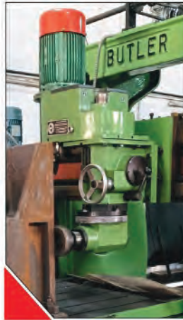
Right Angle Milling Attachment On Milling Head, Virtually Adds Floor Boring Capability To An Used Planer.
