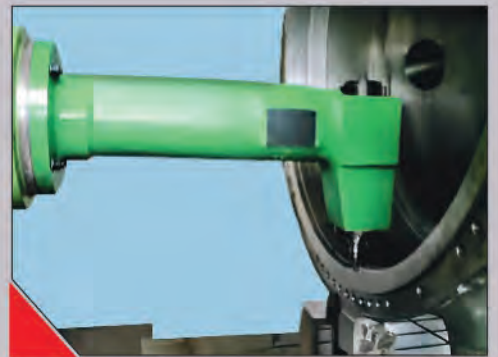
Reach Extended Right Angle Attachment Virtually Increases The Stroke Length Of A Floor Borer & Facilitates Maching In Inaccessible Pockets.
