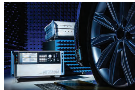
NXP has chosen the R&S RTS radar test system to verify their radar sensor reference design based on the industry's first 28 nm RFCMOS one-chip radar SoC.
