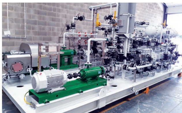
The Plenty Triro is the preferred pump for API 614 oil systems and can be used on a wide variety of compressor, turbine, gearbox, pump seal oil, and sealing system circulation systems.
