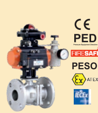
Ball Valves Size: From 15mm to 200mm Bodies: CF8, CF8M with SS 316 Ball Seat Material PTFE/Delrin. Model-2390F
