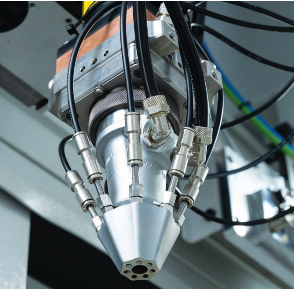
Structure of the laser tool: The coating material is fed in as a powder and fused to the component surface using a laser process.
