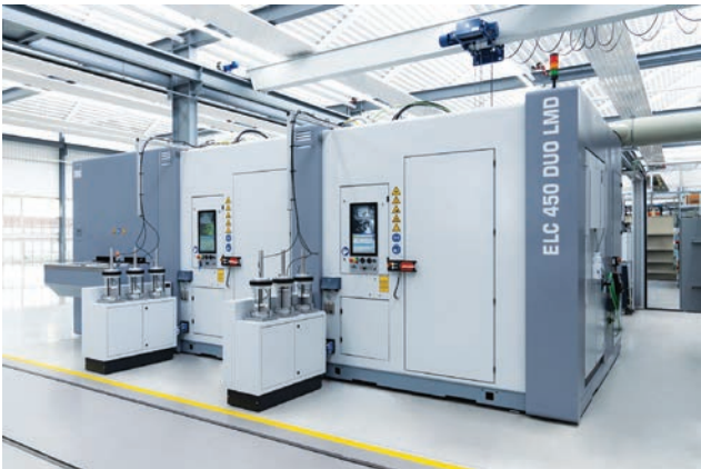
The ELC 450 DUO LMD with two process modules enables increased productivity in the hard coating of brake discs.
