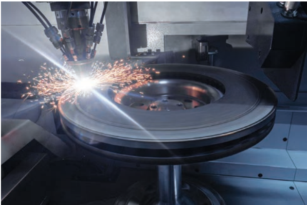
Laser deposition welding is used to apply a hard coating that protects brake discs from corrosion and wear.
