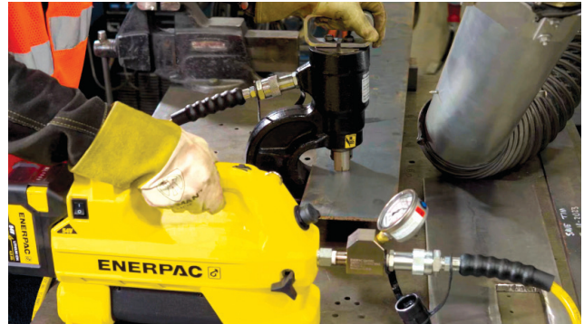
Punching holes using the Enerpac SC-Series portable hydraulic pump
