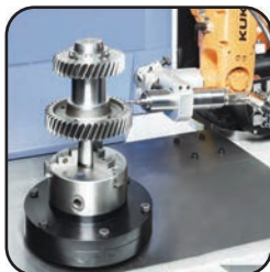
Robotic Deburring of a Cluster-Gear, using a SycoTec Spindle
