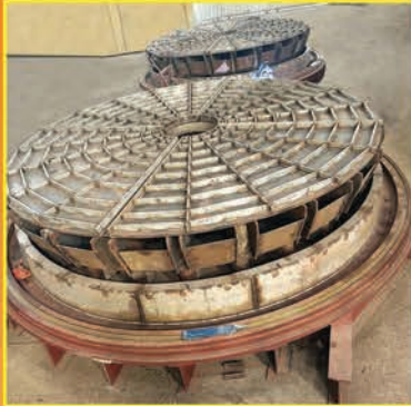
Base for 85 Ton Furnace for wire in Bobbins
