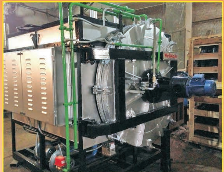
Batch Type Muffle Furnace with Protective Atmosphere
