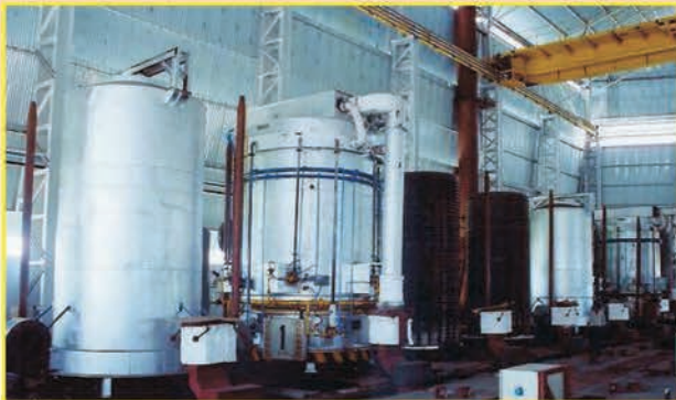
80 Ton Bell Type Bright Annealing Furnace
