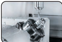
Workpiece in Chuck being machined with SycoTec Spindle
