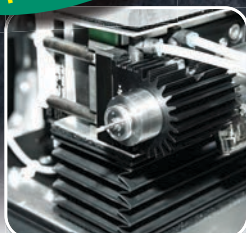
Internal Grinding using a SycoTec Spindle
