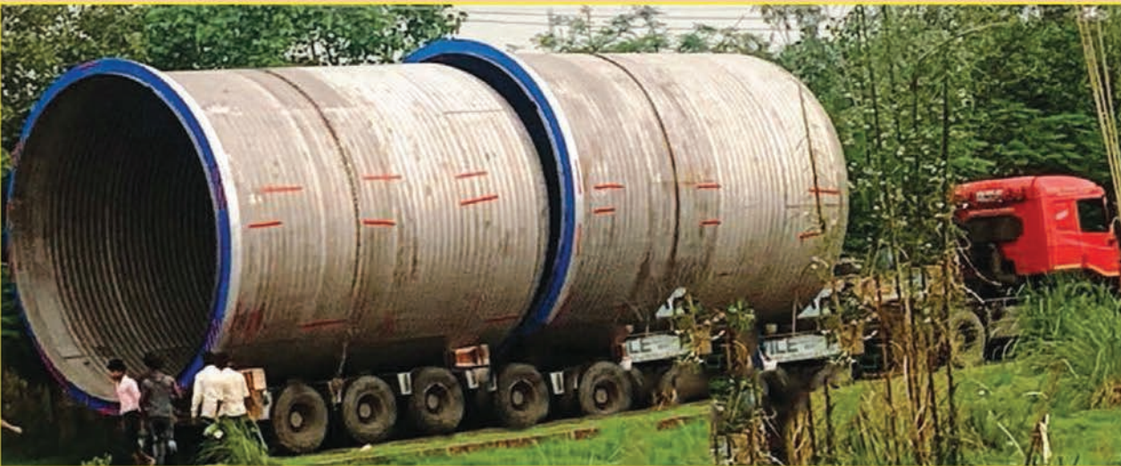
Inner Cover / Retort of 4800 mm ID x 7000 mm Height
