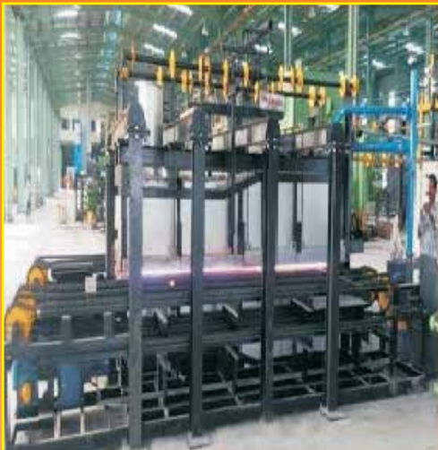
Conveyorised Heating Furnace
