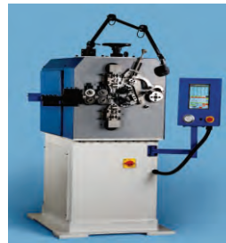
4-Axis CNC Spring Coiling Machine (upto 4.0 mm)
