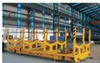
Pipe and Billet Transfer Car
