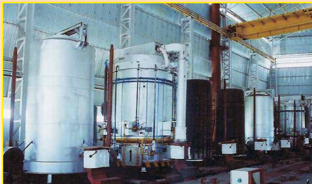
80 Ton Bell Type Bright Annealing Furnace
