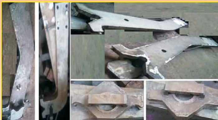
SS 316 L Grade Fabricated Sink Roll and Stabilizer Roll Arms and Bush Housings for Rolls of Galvanising Line.
