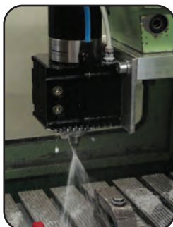
SycoTec Spindle as a 5th Axis for VMC (Vertical Machining Centre)
