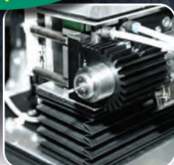
Internal Grinding using a SycoTec Spindle
