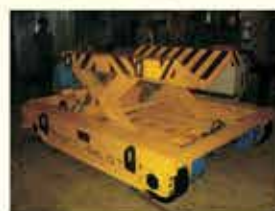
Transfer Car with Scissor Lift
