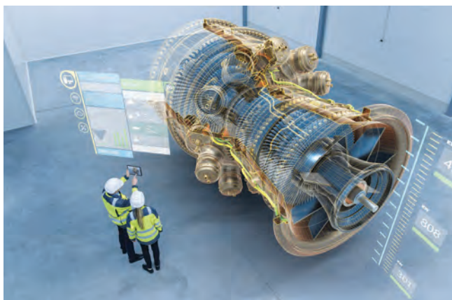
Digital Twin of gas turbine
