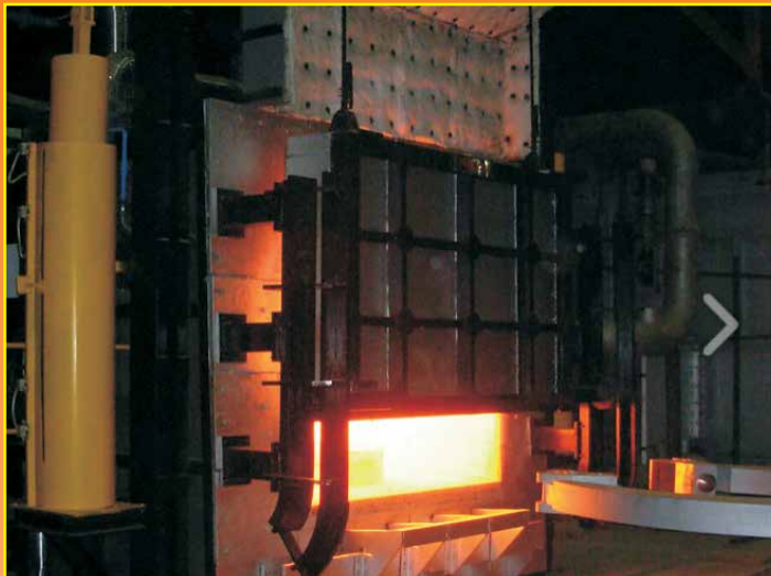
20 Ton/batch capacity Oil Fired Chamber Furnace for Forging with \pm 3 degree C Temperature Control.
