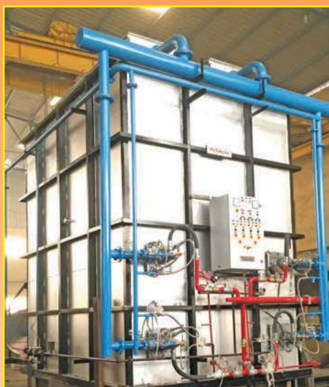
60 Ton Capacity Dual Fuel Fired Sheet Annealing Furnace
